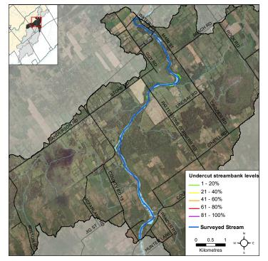
Figure 11 Undercut stream banks along Kemptville Creek Oxford Mills catchment
