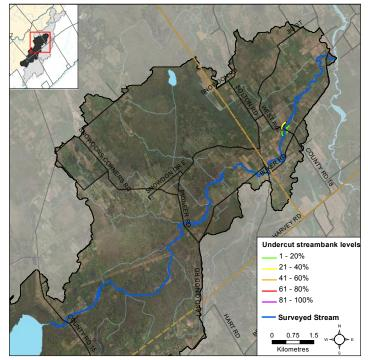
Figure 11 Undercut stream banks along North Branch
