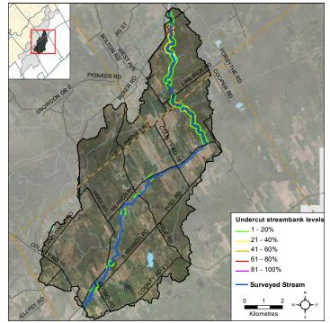
Figure 11 Undercut stream banks along South Branch
