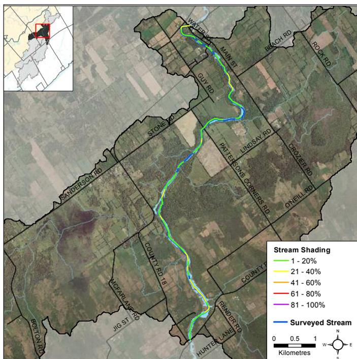
Figure 12 Stream shading along Kemptonville Creek Oxford Mills catchment
