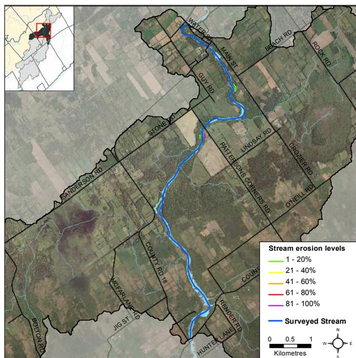
Figure 10 Erosion along Kemptville Creek Oxford Mills catchment
